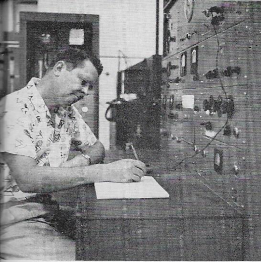
The mass spectrometer is supplying for Ed Beck's record a molecular-weight endorsement of another gas sample's worthiness.
